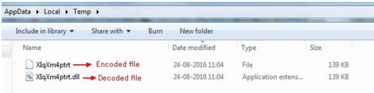
Fig 3. The downloaded encoded file and the respective DLL file obtained after decoding.
